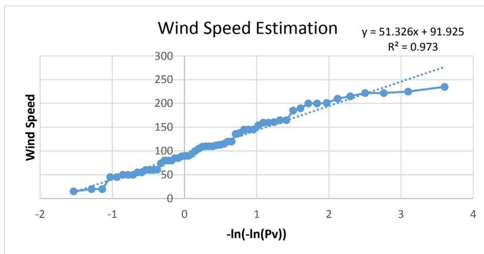
Figure 4.3: Wind speed estimation by plotting wind speed vs  $-\ln(-\ln(Pv))$ ;  $Pv$  is Gringorten estimation of Probability
